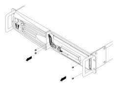
4. Remove the four retaining screws.
